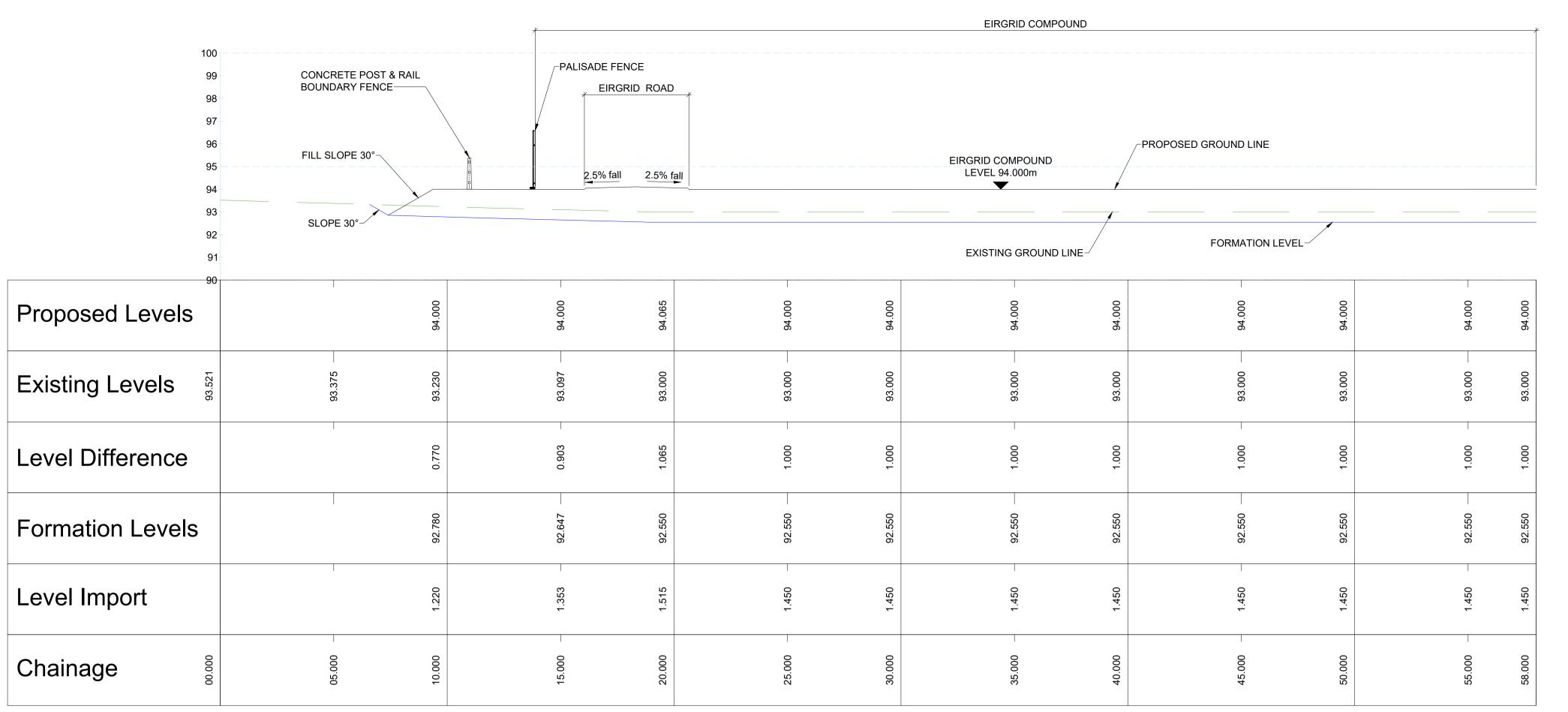
SECTION B - PART 1 CH0.0M TO 58.0M SCALE H 1:125, V 1:125
